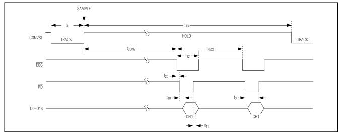
Figure 5. Read During Conversion—Two Channels Selected, Internal Clock
