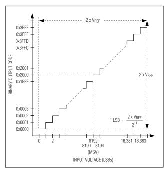
Figure 11. 0 to +5V Unipolar Transfer Function
