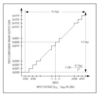
Figure 10. ±5V Bipolar Transfer Function
