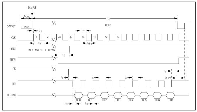
Figure 7. Reading After Conversion—Eight Channels Selected, External Clock
