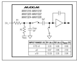
Figure 2. Typical Input Circuit
