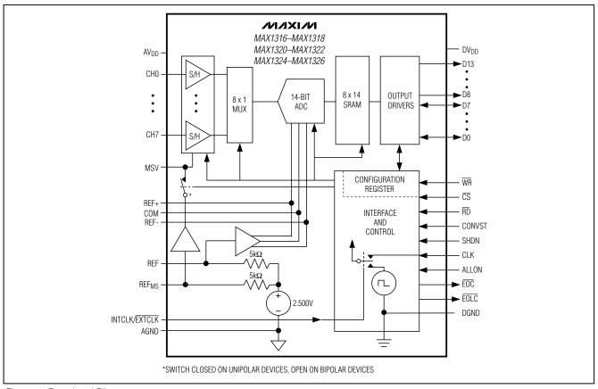
Figure 1. Functional Diagram
