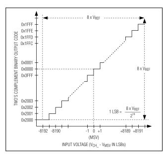
Figure 9. ±10V Bipolar Transfer Function
