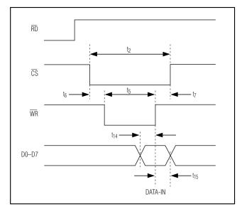
Figure 4. Write Timing
