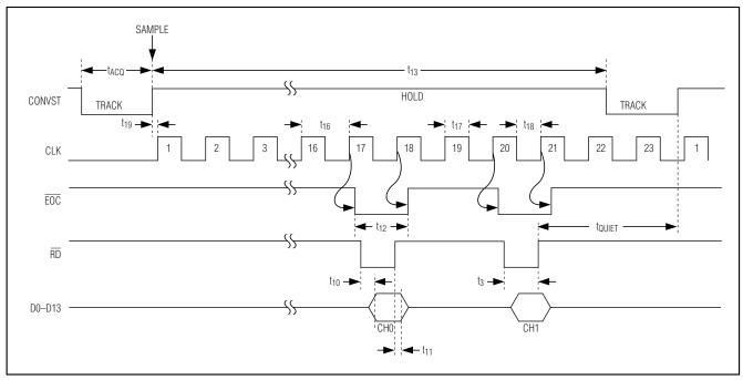
Figure 6. Read During Conversion—Two Channels Selected, External Clock
