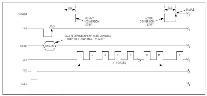
Figure 3. Software Channel Wake-Up Timing (ALLON = 0)
