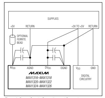
Figure 8. Power-Supply Grounding and Bypassing
